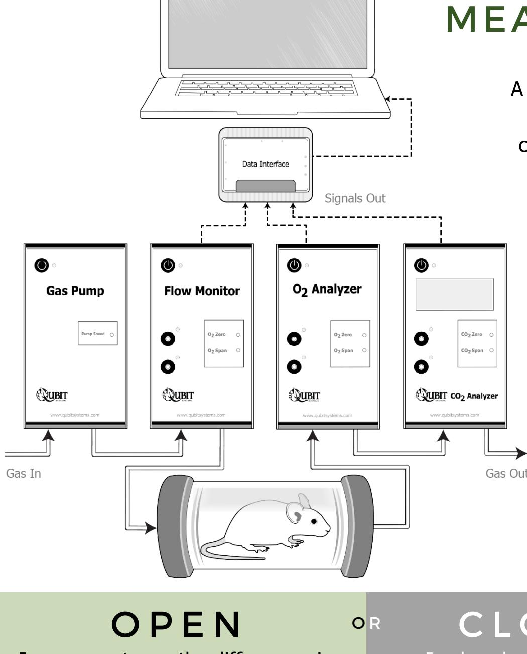
A respirometry system typically includes a chamber in which the sample is accommodated.
